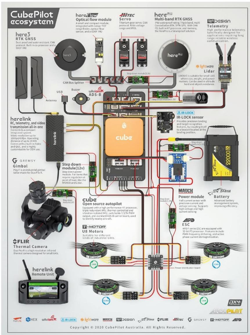
Additionally, the Pixhawk manages various flight modes, offering versatility in performance ranging from stabilized flight to autonomous waypoint navigation. Connected to the Pixhawk are an array of indispensable components that collectively contribute to the drone's seamless operation. The GPS Module (Here3+) provides indispensable positioning data, allowing for accurate navigation and precise waypoint tracking. Telemetry Radios establish a vital communication link with the ground
