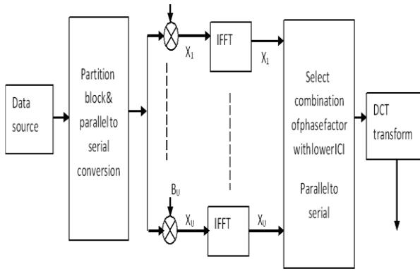
Fig 1 Basic blocks of proposed PTS, DCT-SLM technique
