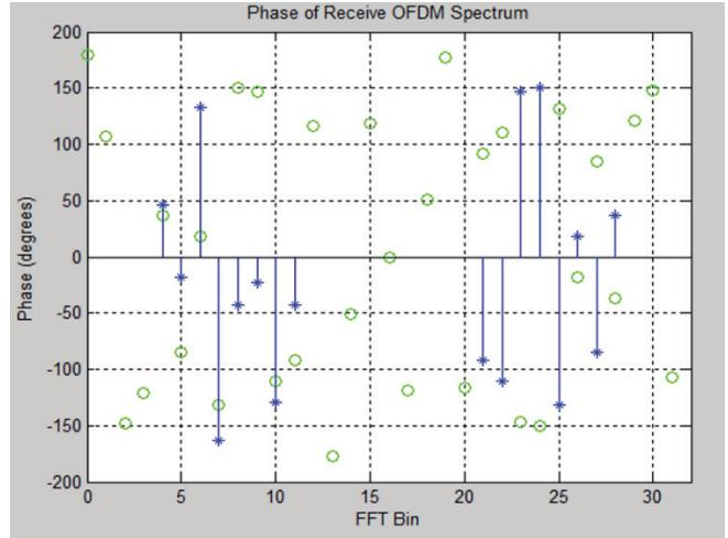
Fig 4 16-PSK OFDM signal & its phases
