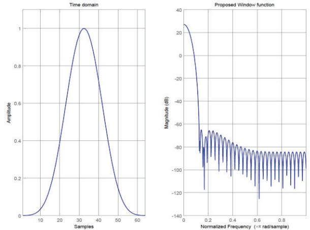
Fig 5 Window function in this work
