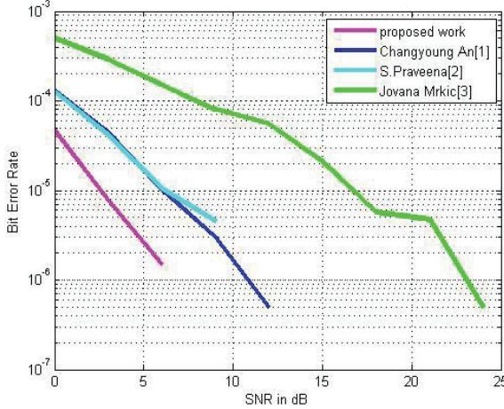
Fig 7. BER obtained when 4PSK modulation comparative observation
