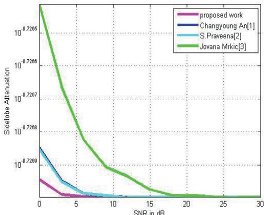
Fig 8 Attenuation in Sidelobe comparison for 50Hz test signal with 4-PSK modulation and different amounts of noise
