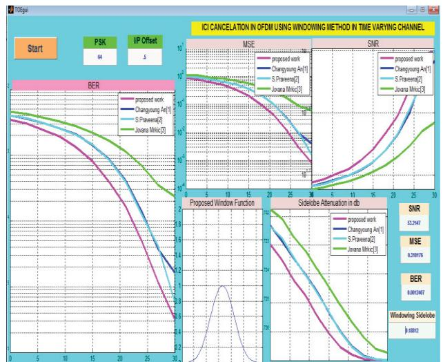
Fig 6. MSE, BER, attenuation in sidelobe, SNR observed for 50Hz test signal with 64-PSK modulation and different amounts of noise
