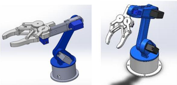
Figure-2: Installation of Servo Motors (Some were enclosed inside the body)
