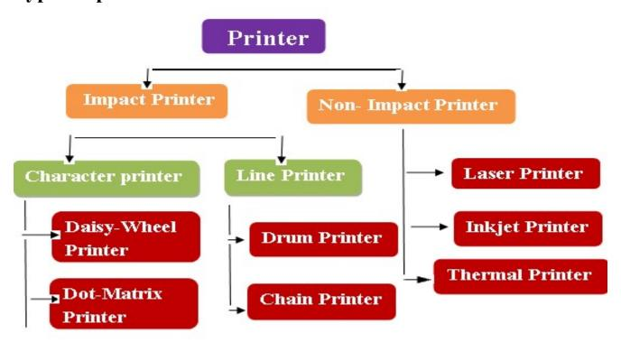
**Impact Printer:**—It is a type of printer that works by direct contact of an ink ribbon with paper. These printers are typically loud but remain in use today because of their unique ability to function with multipart forms. An impact printer has mechanism similar to a typewriter. Example of Impact Printers: Dot-matrix printers, Daisy-wheel printers, and line printers.
