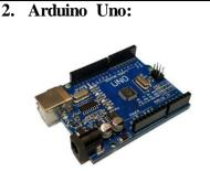
Arduino Uno is a microcontroller board based on the ATmega328P (datasheet). It has 14 digital input/output pins (of which 6 can be used as PWM outputs), 6 analog inputs, a 16 MHz ceramic resonator.
