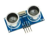
Ultrasonic sensors are electronic devices that determine a target's distance. They work by emitting ultrasonic sound waves and converting those waves into electrical signals. Furthermore, ultrasonic travel at a faster rate than audible sounds. Therefore, ultrasonic sensor work involves sound waves to find the distance to an item.
