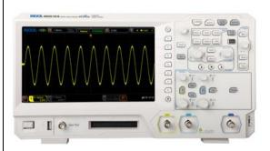
A digital storage oscilloscope (DSO) is an oscilloscope which stores and analyses the input signal digitally rather than using analog techniques. It is now the most common type of oscilloscope in use because of the advanced trigger, storage, display and measurement features which it typically provides.
