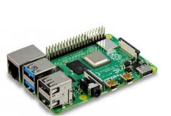
The Raspberry Pi is a small, low-cost computer that is about the size of a debit card. It has a processor, memory, and graphics driver, and can connect to a TV or computer desktop using a keyboard and mouse.
