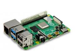
The Raspberry Pi is a small, low-cost computer that is about the size of a debit card. It has a processor, memory, and graphics driver, and can connect to a TV or
