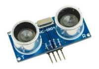
Ultrasonic sensors are electronic devices that determine a target's distance. They work by emitting ultrasonic sound waves and converting those waves into electrical signals. Furthermore, ultrasonic travel at a faster rate than audible sounds. Therefore, ultrasonic sensor work involves sound waves to find the distance to an item.
